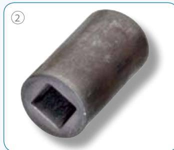
Hot forged in the forging press.
